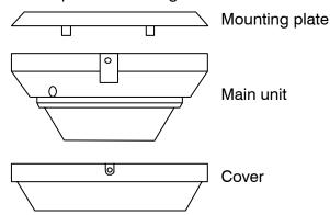
3. Connect the wires according to the diagram of the desired control mode. Replace the main unit, then test can be conducted.
