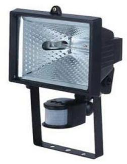
The infrared induced lamp has an infrared detector within it. When the thermal body moving in the darkness the detector will light the lamp automatically and turn off after a period of time set in advance.
